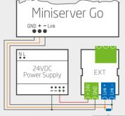
Keep in mind that GND needs to be connected to the ground of the 24V Power. 120Ω termination resistor
